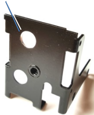
To 6: drill hole up to 10mm
